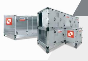
WIZARD air handling units are specially designed to cater to any installation needs. The range consists of 23 standard sizes, with air flow ranges varying from 1,000 to 115,500 m<sup>3</sup>/h, and face air speed through the coils of 2,5 m/s. WIZARD can be combined with a wide range of accessories, making it the most suitable unit not only for standard applications but also for special ones.
